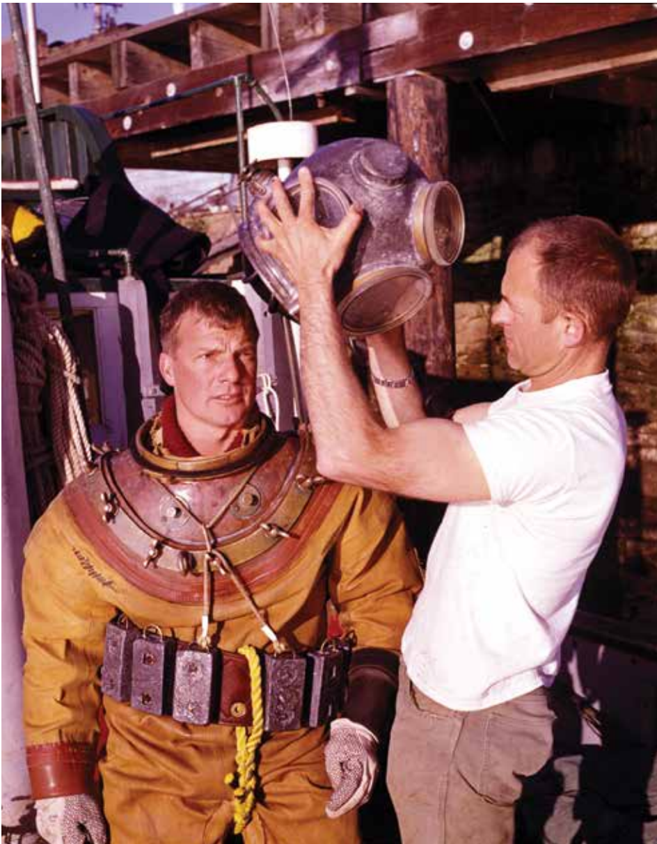
1964. Bev Morgan being dressed in by Bob Christensen during construction on the Trans-Pacific telephone cable. This “Whatever it takes to get the job done,” diving is exemplified by the way Morgan’s weight belt is rigged and the period Japanese helmet bonnet being attached to a turn of the century, or earlier, Canadian breastplate Morgan is wearing.
