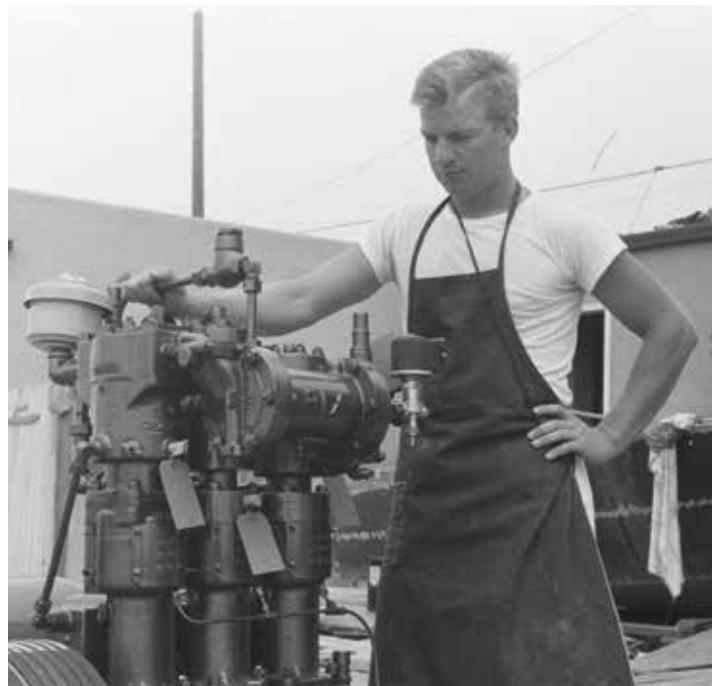
Bev Morgan looking over the new Rix water lubed high pressure compressor in 1955. Rear yard of Dive 'N Surf.
