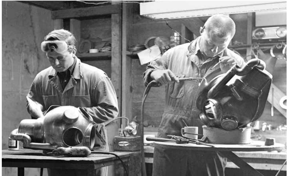
1966. Bev Morgan and Bob Kirby constructing two bonnets of Kirby's design of commercial helium recirculator helmets, from an order of four helmets. One of the actual four helmets is shown on page 11 of The Helmets That Launched Commercial Mixed Gas Diving , Journal of Diving History , issue 91, and can currently be seen on display in Santa Barbara Maritime Museum.
